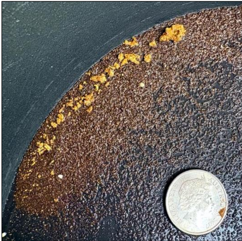
Figure 9: Visible Gold recovered from panning the bulk 1m sample for the interval 37-38m in Musketeer drill hole INRC25073, which reported 1m at 356g/t Au. Coin for scale is approximately 20mm in diameter 14 .
