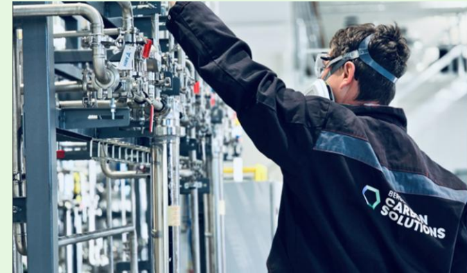
The separation unit separates the carbon from electrolyte
