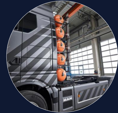
MAN hTGX FCEV heavy-duty truck with 200 deliveries in 2025 Range: 600 km Refuel time: 15 min or less
