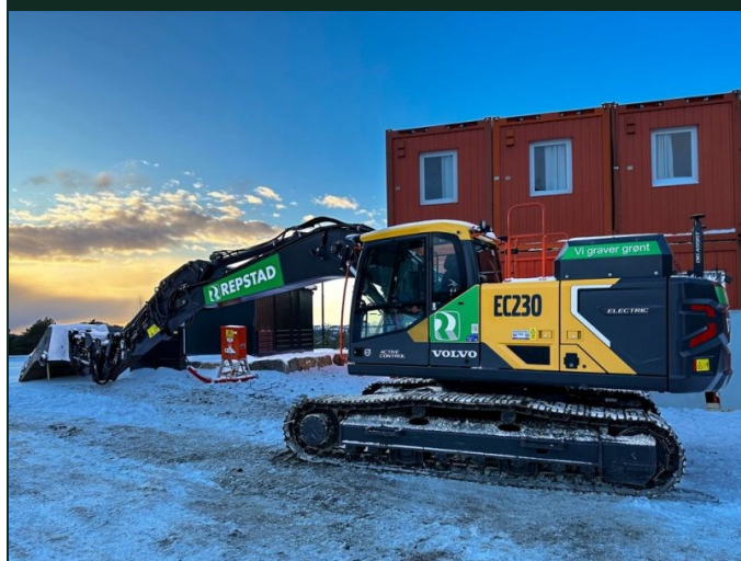
Electric excavator purchased by Repstad Anlegg AS in 2023
