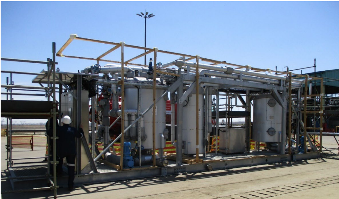
Photo: Cambi's THP pilot unit for the commercial trial at Secunda Operations (courtesy of Sasol)
