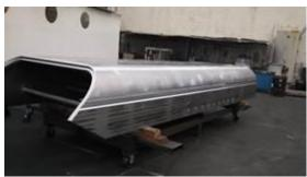
Finished formed and machined hull
