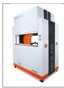
The MiniLAB I 6 GHz OTA uses proven electronic scanning technology to evaluate the electromagnetic field on a full sphere surrounding the antenna. Power is measured using an array of bipolar probes that scan the object within a few seconds.
