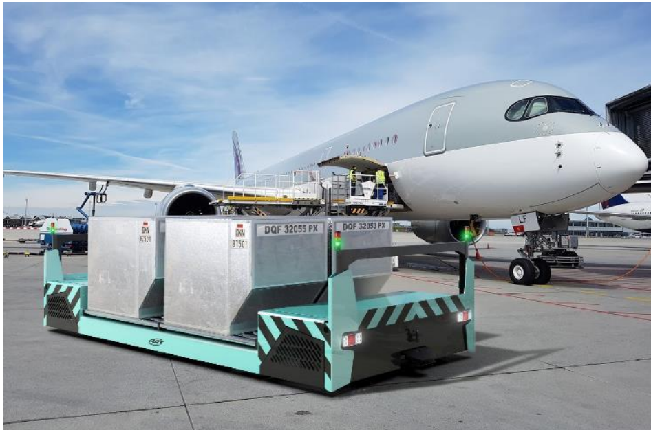
AAT (Autonomous Airport Transporter) FULL ELEC en configuration double UC et TANDEM
