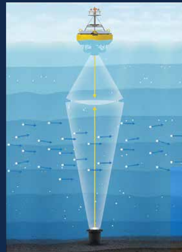
Example of a high-frequency ADCP (buoy-mounted) used in conjunction with a low-frequency ADCP (bottom-mounted) to cover the full water column.
